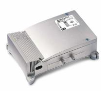
1-input (III+DAB+UHF) multiband TV indoor amplifier with 43dB gain and up to 125dBµV output level on UHF band, separate amplification with independent level adjustment (20dB) for each band and low noise figure. T2 technology with UHF cut band for LTE 4G @790MHz and 5G @694MHz.
